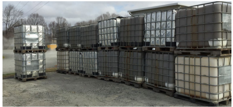
BEFORE (above): Wastewater chemicals were stored in totes. This presented concerns with spills, storm water and safety.
